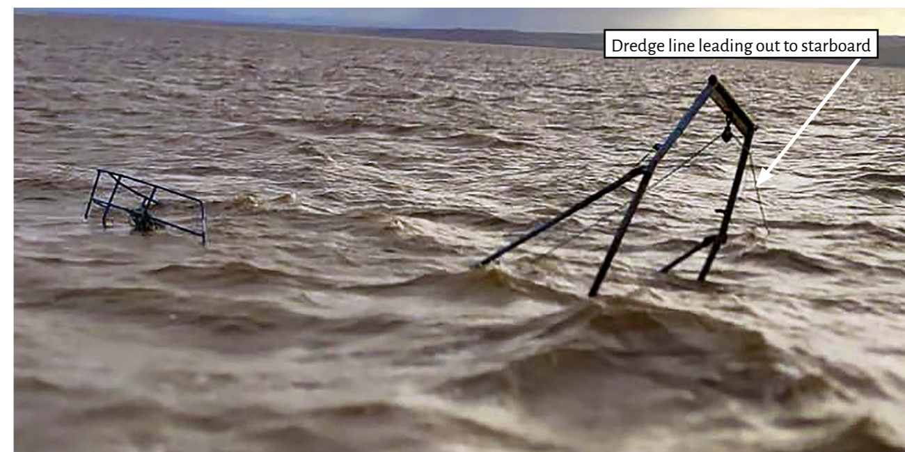
Figure 1: The dredger capsized to starboard with only the bow rails and dredging gantry visible
