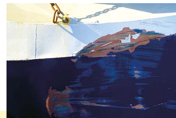
Figure: Damage to the beam trawler's bow
