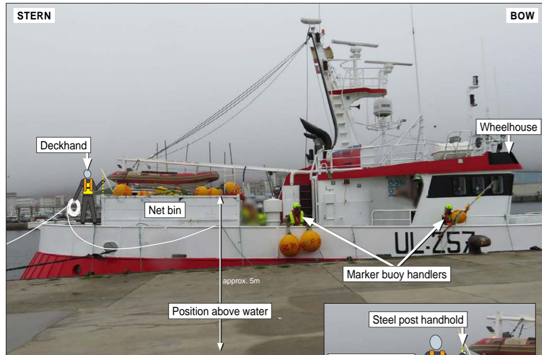
Reconstruction, showing the positions of the deckhands during the final phase of shooting the net
