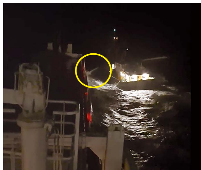
Figure 1: Video still showing the bulk carrier hitting the fishing vessel's deployed derrick arm
