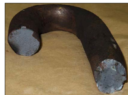
Figure 2: Failed chain link on Honeybourne III
